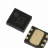
XC6121A218ER-G Torex Semiconductor Ltd IC WATCHDOG TIMER 6-USP
