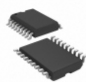
PIC16C711-20I/SO Microchip Technology IC MCU 8BIT 1.75KB OTP 18SOIC
