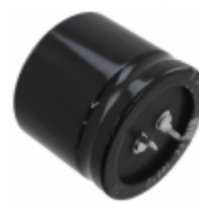
LGR2W151MELC30 Nichicon CAP ALUM 150UF 20% 450V SNAP
