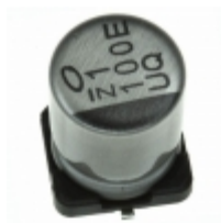
UUQ0J221MCL1GS Nichicon CAP ALUM 220UF 20% 6.3V SMD
