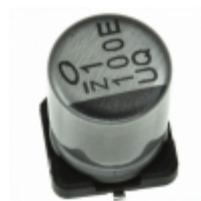
UUQ0J331MCL6GS Nichicon CAP ALUM 330UF 20% 6.3V SMD
