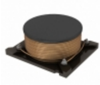
AX97-40820 Triad Magnetics FIXED IND 82UH 2.2A 120 MOHM SMD
