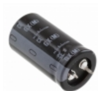
LGX2E471MELZ40 Nichicon CAP ALUM 470UF 20% 250V SNAP
