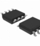
TC4428EOA Micrel / Microchip Technology IC MOSFET DVR 1.5A DUAL HS 8SOIC
