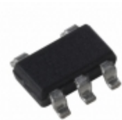
MIC5256-2.6BM5-TR Microchip Technology IC REG LDO 2.6V 0.15A SOT23-5
