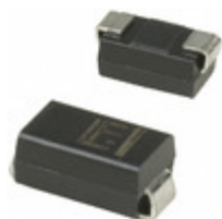
SMAJ33C Littelfuse Inc. TVS DIODE 33VWM 55.97VC SMA
