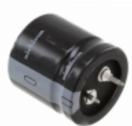
LQS2W101MELA25 Nichicon CAP ALUM 100UF 20% 450V SNAP
