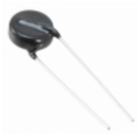
ERZ-E11A511 Panasonic Electronic Components VARISTOR 510V 6KA DISC 13MM
