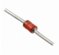
MXP4KE350CA Microsemi Corporation TVS DIODE 300VWM 482VC DO41
