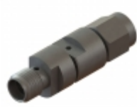
SF0930-6200-09 Amphenol SV Microwave ATTENUATOR 18GHZ 9DB 50 OHM SMA
