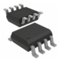
AD736JR-REEL7 Analog Devices Inc. IC AC RMS TO DC CONV 5V 8-SOIC
