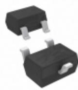
BSS138W L6327 Infineon Technologies MOSFET N-CH 60V 280MA SOT-323
