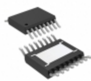
LT3697IMSE#PBF ADI (Analog Devices, Inc.) IC REG BUCK ADJ 2.5A 16MSOP
