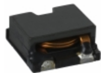
CEP125-1R0MC-HD Sumida America Components Inc. FIXED IND 1UH 16.5A 2.5 MOHM SMD
