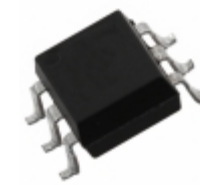
EL3063S(TA) Everlight Electronics Co Ltd OPTOISOLATOR 5KV TRIAC 6SMD
