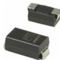
P4SMA200 Littelfuse Inc. TVS DIODE 171VWM 287.7VC SMD
