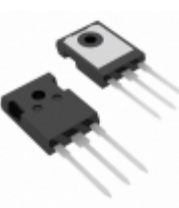
DSB80C45HB IXYS DIODE ARRAY SCHOTTKY 45V TO247AD
