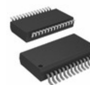
PIC18LF26K80-I/SS Microchip Technology IC MCU 8BIT 64KB FLASH 28SSOP
