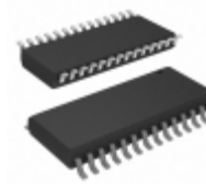
PIC18LF26K80-I/SO Microchip Technology IC MCU 8BIT 64KB FLASH 28SOIC
