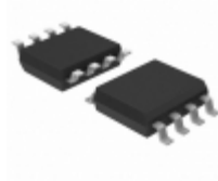
MAX6198BESA+ Maxim Integrated IC VREF SERIES 4.096V 8SOIC
