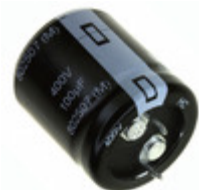
EET-HC2D102BA Panasonic Electronic Components CAP ALUM 1000UF 20% 200V SNAP
