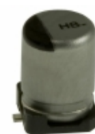
EEV-HB0J220R Panasonic Electronic Components CAP ALUM 22UF 20% 6.3V SMD
