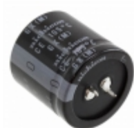
LGX2W331MELC35 Nichicon CAP ALUM 330UF 20% 450V SNAP
