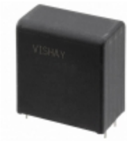
MKP1848C56012JP4 Vishay BC Components CAP FILM 6UF 5% 1.2KVDC RAD 4LD
