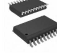
PIC24FV16KA301-I/SO Microchip Technology IC MCU 16BIT 16KB FLASH 20SOIC
