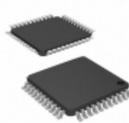
PIC24FV08KM204T-I/PT Microchip Technology IC MCU 16BIT 8KB FLASH 44TQFP
