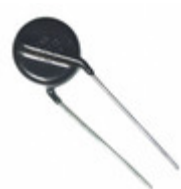
ERZ-E10F681 Panasonic Electronic Components VARISTOR 680V 4.5KA DISC 12.50MM
