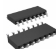
LT1721CS#PBF Linear Technology IC COMP R-RINOUT QUAD 16-SOIC
