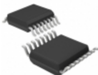
LT6207IGN#PBF Linear Technology IC OPAMP VID QUAD 100MHZ 16- SSOP
