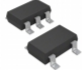
ADP166AUJZ-2.3-R7 Analog Devices Inc. IC REG LDO 2.3V 0.15A 5TSOT
