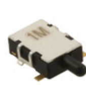
CL-DA-1CB4-A2T Copal Electronics Inc. SWITCH DETECTOR SPST-NO 100MA
