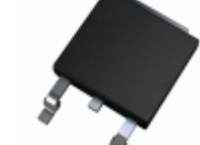
MJD50T4 STMicroelectronics TRANS NPN 400V 1A DPAK
