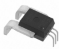
ACS758KCB-150U-PFF-T Allegro MicroSystems, LLC SENSOR CURRENT HALL 150A DC
