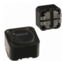
DRQ127-6R8-R Eaton INDUCT ARRAY 2 COIL 7.387UH SMD
