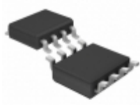
LTC1682IS8-5#TRPBF ADI (Analog Devices, Inc.) IC REG SWITCHD CAP 5V 50MA 8SOIC
