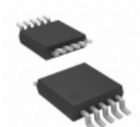
MCP4262-103E/UN Microchip Technology IC RHEOSTAT 10K 2CH 10MSOP
