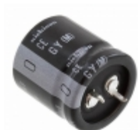
LGY2V101MELA Nichicon CAP ALUM 100UF 20% 350V SNAP
