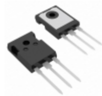
IXGH32N60AU1 IXYS IGBT 600V 60A 200W TO247AD
