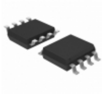
AT25040AN-10SU-1.8 Microchip Technology IC EEPROM 4KBIT 20MHZ 8SOIC
