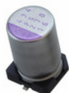
16SVPG47M Panasonic Electronic Components CAP ALUM POLY 47UF 20% 16V SMD
