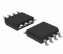
MCP6V01T-E/SNVAO Micrel / Microchip Technology IC OPAMP CHOPPER 1.3MHZ 8SOIC
