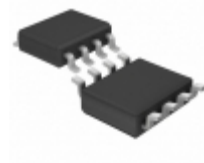
LTC1504CS8-3.3#PBF Linear Technology / Analog Devices IC REG BUCK 3.3V 0.5A SYNC 8SOIC
