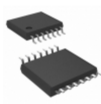
ADTL084ARUZ Analog Devices Inc. IC OPAMP JFET 5MHZ 14TSSOP
