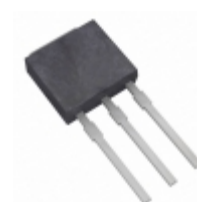
RFD14N05L Fairchild/ON Semiconductor MOSFET N-CH 50V 14A I-PAK
