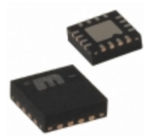
MIC68400-2.5YML-TR Microchip Technology IC REG LDO 2.5V 3A 16MLF
