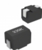
CM453232-331KL Bourns Inc. FIXED IND 330UH 85MA 14 OHM SMD
