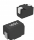
CM453232-390KL Bourns Inc. FIXED IND 39UH 150MA 4.5 OHM SMD
