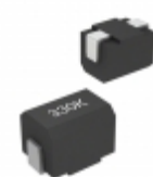
CM453232-3R3JL Bourns Inc. FIXED IND 3.3UH 355MA 800 MOHM
