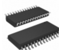
PIC16C57T-LPE/SO Microchip Technology IC MCU 8BIT 3KB OTP 28SOIC
