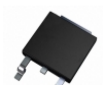
IRFR9024NTRR Infineon Technologies MOSFET P-CH 55V 11A DPAK
