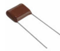
ECQ-E4334JF3 Panasonic Electronic Components CAP FILM 0.33UF 5% 400VDC RADIAL
